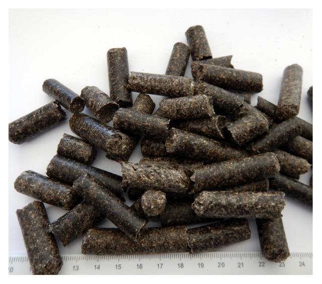
Diameter : 10- 12 mm It is possible to buy either 10 mm or 12 mm or a mixture of both diameters
